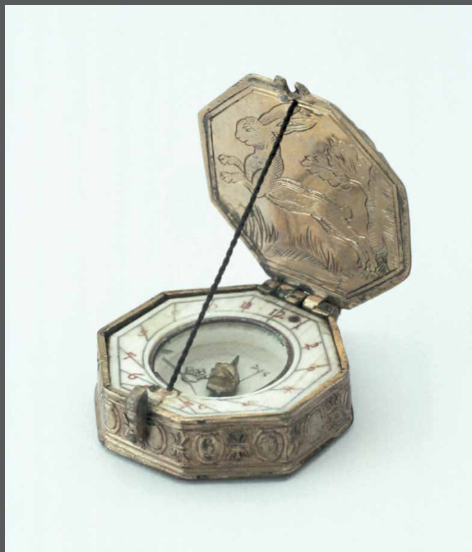
Fig. 15. Lienhart Miller, 1631: horizontal sundial as a ring; 38 × 30 × 28 mm, monogram L.M. (taken from KERN 2010, Fig. 28, description 496–497).
