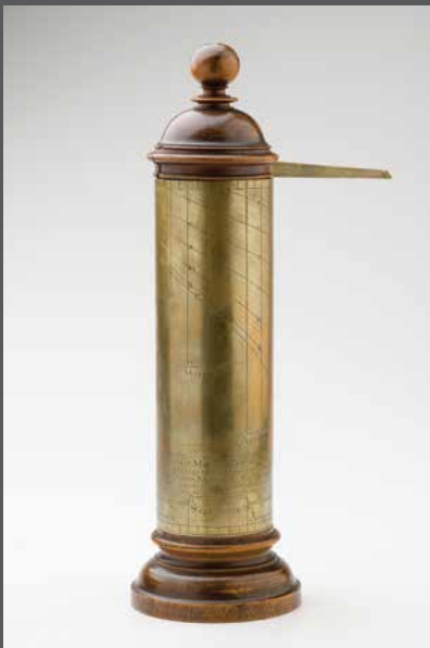
Fig. 5. Table pillar dial, Bohemia, 1745, total height 310 mm, height of brass cylinder 191 mm, cylinder diameter 91 mm. The widely used travelling pillar dial was roughly half the size and was held suspended when measuring (stored at the UPM in Prague, Inv. No. 79462; photo © Ondřej Kocourek, UPM in Prague).
